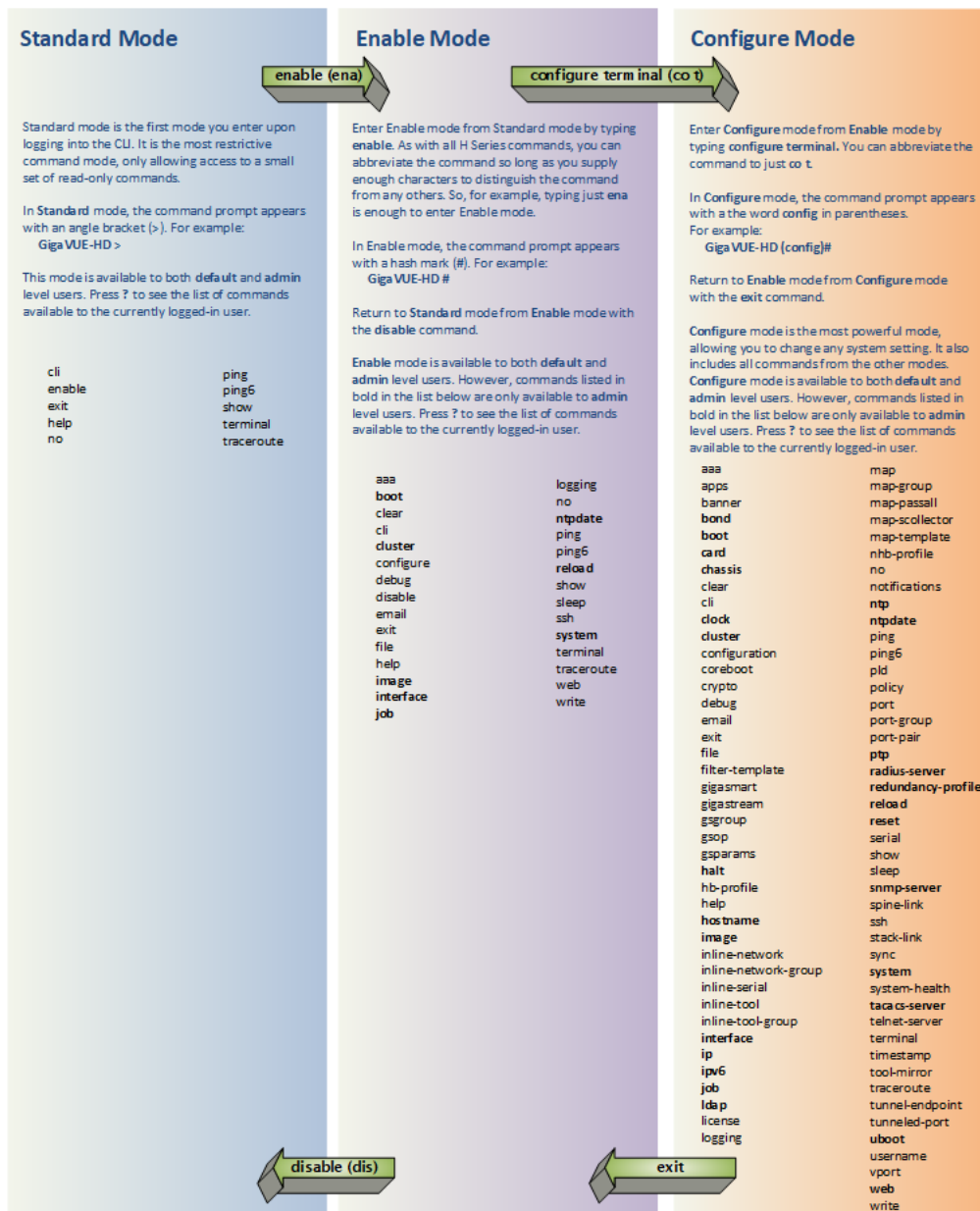
Figure 9 GigaVUE-OS Command-Line Modes
