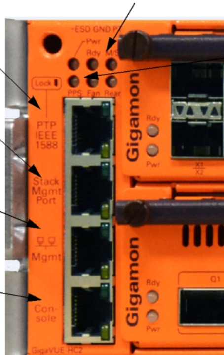
Figure 3 GigaVUE-HC2 Management Ports
